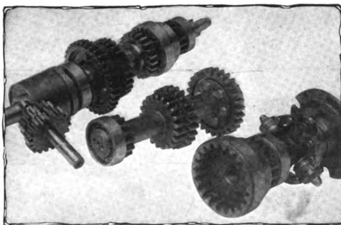
Fig. 14—Three gearshafts and gears in Crossley change-speed set
